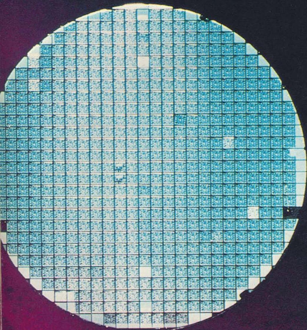
Transistors and circuits are combined on a silicon wafer (above). Subsequently, the wafer is diced into chips.
