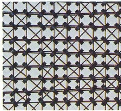
↑ Current-carrying wires that pass through iron oxide cores magnetize them clockwise or counterclockwise. Cores switched from one magnetic state to the other in millionths of a second. One magnetic direction represents a zero, the other, a one in the computer's binary code. Inventors outside IBM originally developed the donut-shaped cores for memory, and IBM perfected the method for making them. The company adapted pill-making machinery to produce them by the millions.
